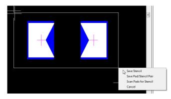
As can be seen from the image above, the Pad / Stencil Pair can be saved directly from UI by creating a selection box while the Shift key is depressed. This allows the original pad pattern and the final stencil pattern to be saved to the database (or file folder) currently in use. The user can create multiple folders to store patterns based on
